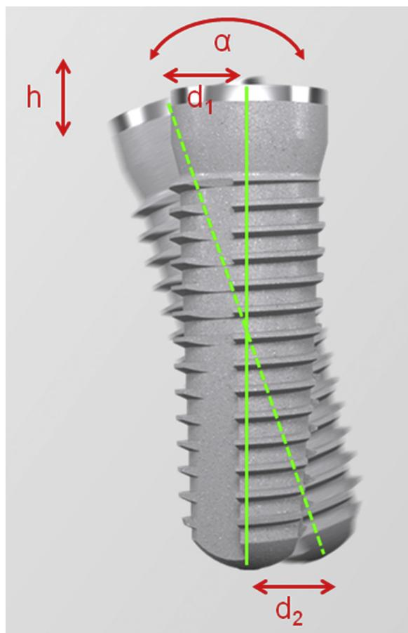
Fig. 4. Calculated deviations: Height ( $h$ ),  $d_1$  (implant neck) and  $d_2$  (implant apex) in millimeters, and angle ( $\alpha$ ) between implant axes [°].
